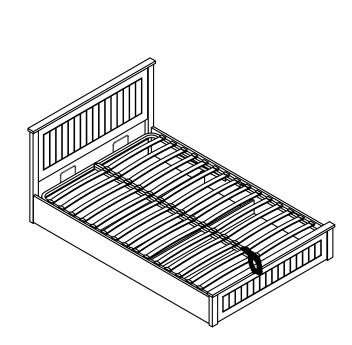
Push x2 mattress stoppers (10) into the holes in the metal frame, they should go all the way through the upper & lower metal sections.
